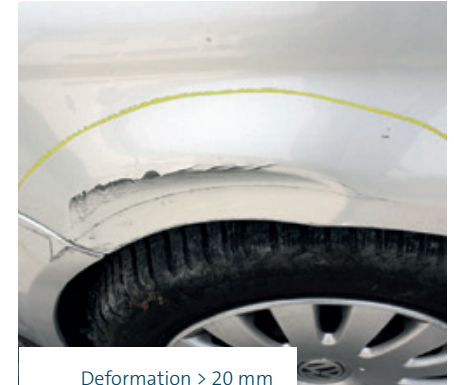
Deformation &gt; 20 mm
